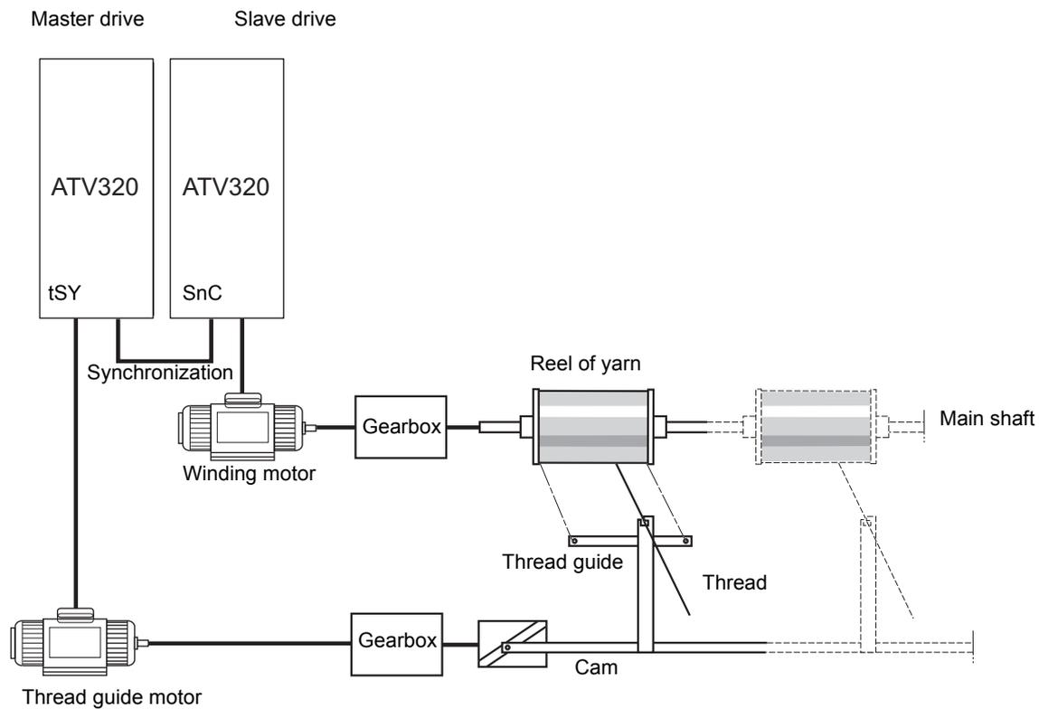
The Counter wobble function is used in certain applications to obtain a constant yarn tension when the Traverse control function is producing considerable variations in speed on the yarn guide motor ([\[Traverse freq. high\] \(E r H\)](#) and [\[Traverse Freq. low\] \(E r L\)](#), see [\[Traverse freq. high\] \(E r H\)](#) page [242](#)).
