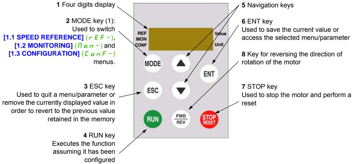
(1) If the drive is locked by a code ([PIN code 1] (Lcd) page 300), pressing the MODE key enables you to switch from the [1.2 MONITORING] (MON-) menu to the [1.1 SPEED REFERENCE] (REF-) menu and vice versa.
