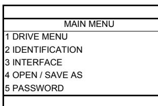
The MAIN MENU appears on the graphic display terminal if you press the ESC key.
