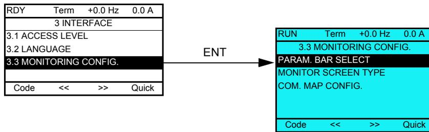
This can be used to configure the information displayed on the graphic display screen during operation.
