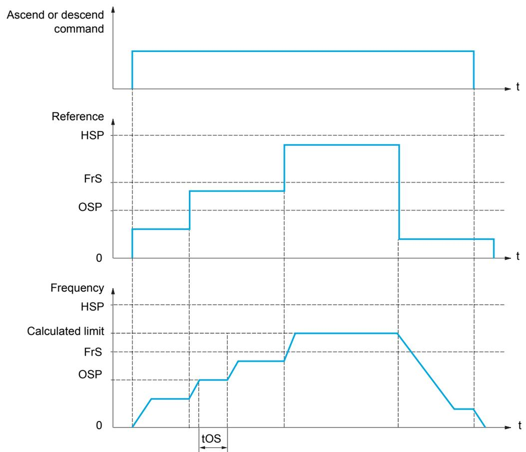
OSP: Adjustable speed step for load measurement
