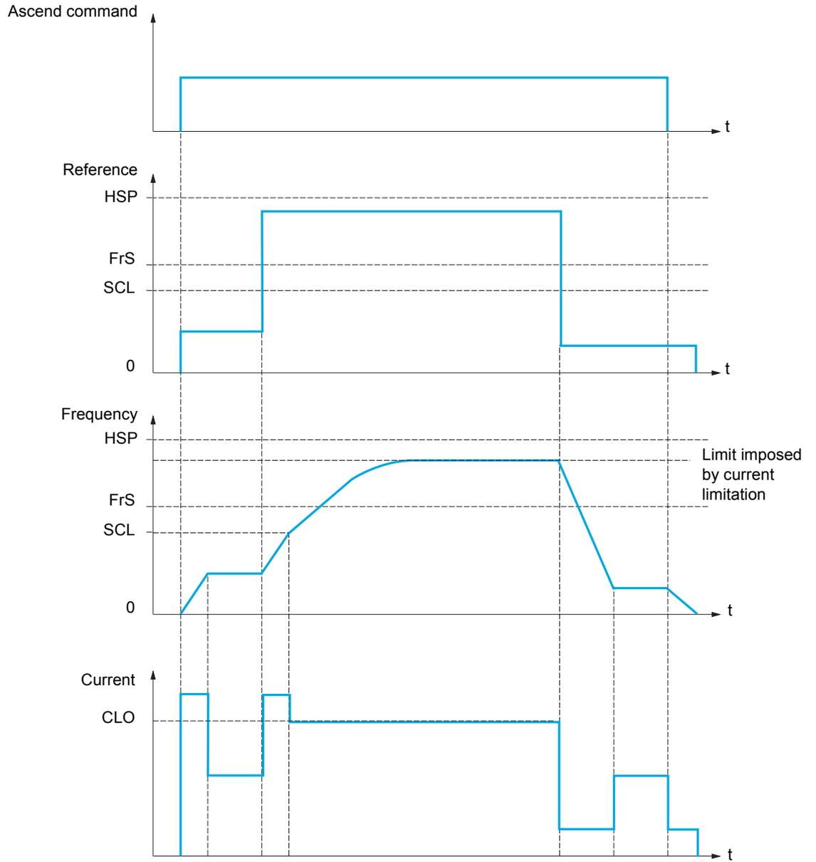
SCL: Adjustable speed threshold, above which current limitation is active
