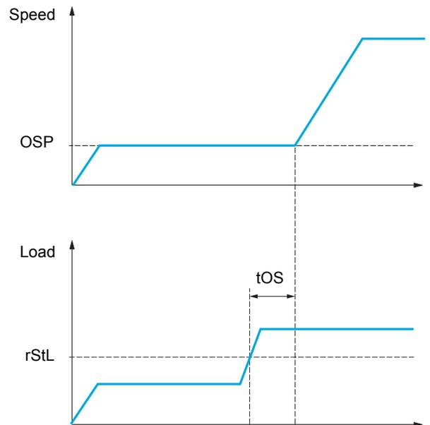
The speed step (OSP parameters) described on page 202 is used to measure the load. The effective measurement cycle will not be triggered until the load reaches the adjustable threshold **[Rope slack trq level] (rStL)**, which corresponds to the weight of the hook.
